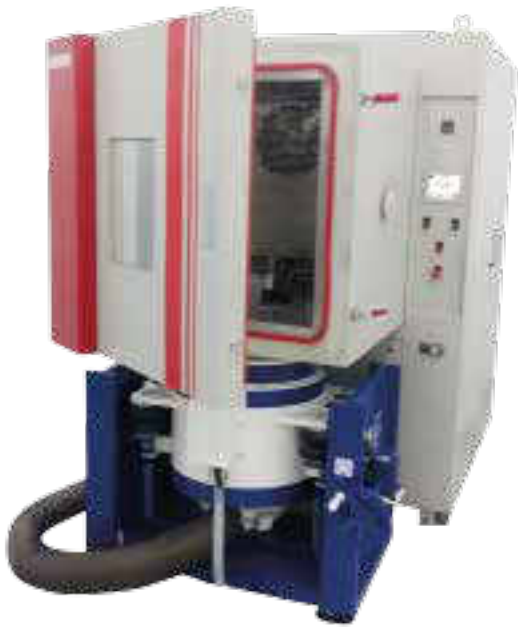
Vibration Combined Climatic Chamber
